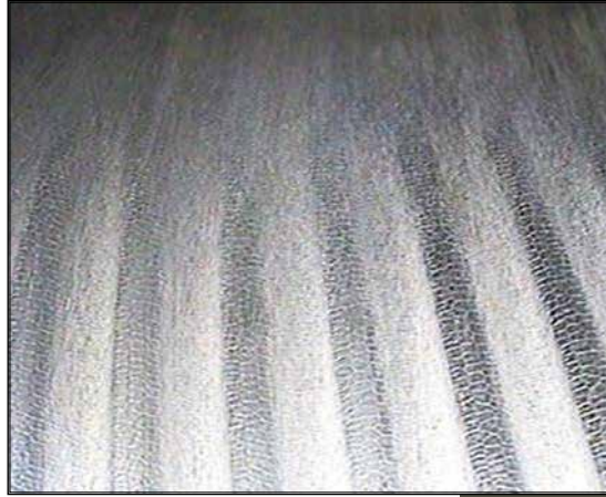
Same 155mm cannon barrel - brand new and towards wear life time
