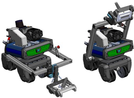
Figure 5: BIKE with ECA probe with lowered (left) and raised (right) actuator arm
