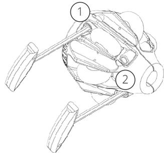
Put the camera in-between the two half shells. The camera head is positioned outside the front of the trolley.
