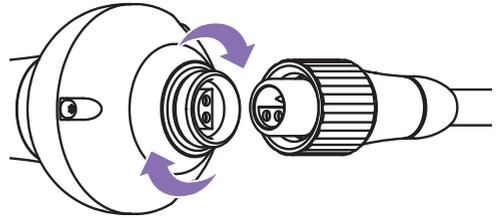
Hand-tighten the screw connection of the plug.
