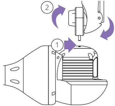
Attach the air pump to the valve of the camera head. Flap the lever of the air pump up in order to fix it to the valve.
