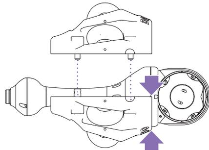
Hand-tighten both screws with the supplied key.
